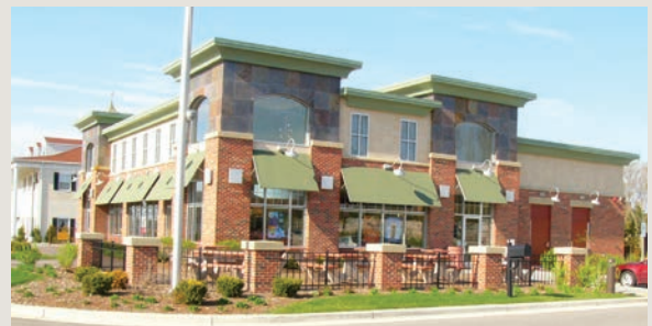
Desired design for a retail building. The color palette includes natural and earth tones. Building has uses brick (primary) and EIFS (secondary), with architectural details that breakdown the facade to human scale. There are varying building planes and heights.
